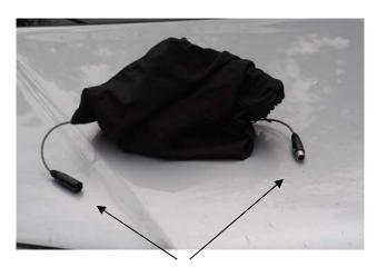
Keep both ends of the cable out of the stuff sack for rapid deployment.
