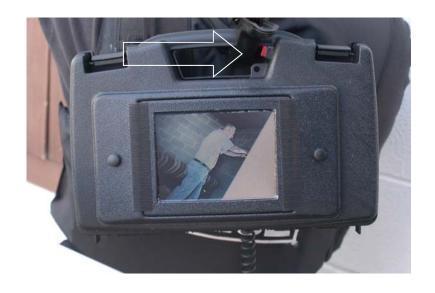
Use the red push-button switch to turn Eagle Vision EV-VS on and off. (We keep it simple!)
