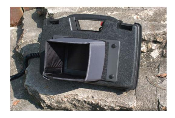
Computer monitors and the Sun do not mix well. Use the sun shade to help you see the picture in the sunlight or to keep the light from the monitor from spreading at night.
