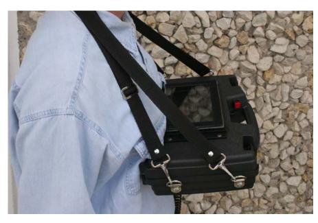
FOR BETTER STABILITY USING THE CHEST MOUNT, CLIP ONE STRAP TO THE TOP "D" RINGS AND ONE STRAP THE BOTTOM "D" RINGS AND ADJUST ACCORDINGLY
