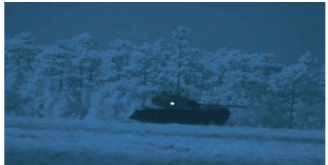
Tank on overcast night with 1,064 Nd:YAG laser spot visible.
